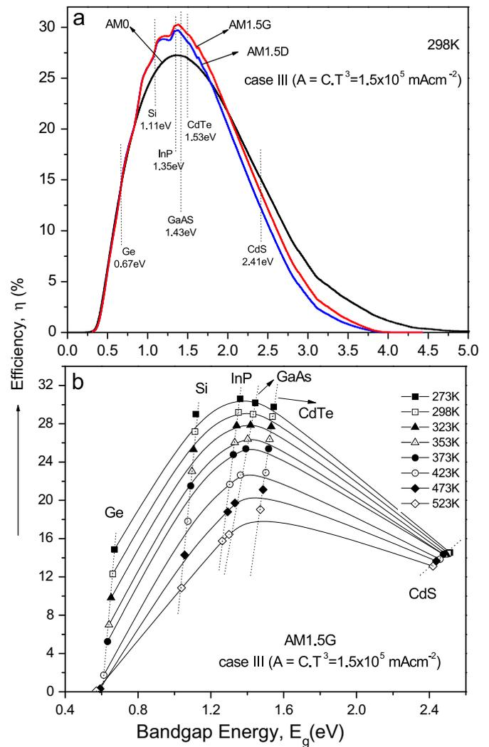
**Fig. 6.** (a) Maximum achievable efficiencies for a single p–n junction solar cell at 298 K as a function of the bandgap energy for the spectra AM0, AM1.5G and AM1.5D. (b) The efficiency of solar cells as a function of bandgap and temperature (case-III) for AM1.5G.
