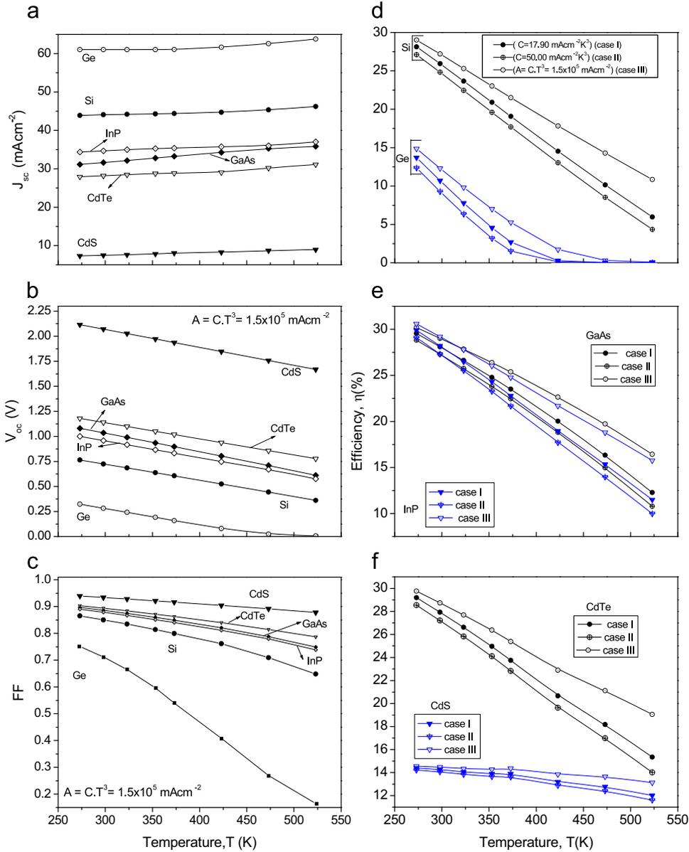
**Fig. 4.** Variations in solar cell performance parameters; (a)  $J_{sc}$ . (b)  $V_{oc}$ . (c) FF. (d)  $\eta$  for Ge, Si (e)  $\eta$  for GaAs, CdTe and (f)  $\eta$  for CdTe and CdS with temperature for solar cells in the temperature range 273 K–523 K. In (b) and (c)  $V_{oc}$  and FF are computed for case (III). In (d–f),  $\eta$  is calculated for three cases (I), (II) and (III), the solid (●) and ‘+’ symbols represent cases (I) and (II) whereas open (○) symbol represents the case (III).
