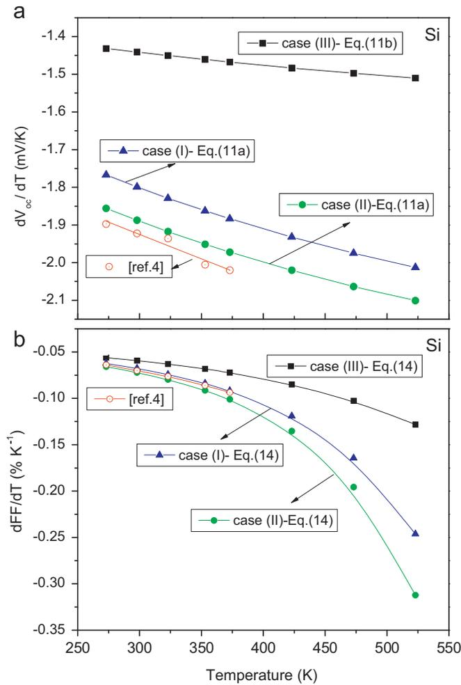
**Fig. 5.** Rate of change of  $V_{oc}$  and FF for Si solar cells (a)  $dV_{oc}/dT$  calculated from Eq. (10a) (cases-I and II) and (10b) (case-III). (b)  $dFF/dT$  calculated from Eq. (14) (cases-I, II and III) in the temperature range 273–523 K along with the values obtained by Fan [4].
