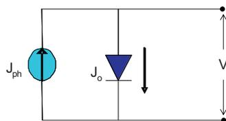
Fig. 1. Equivalent circuit of an ideal solar cell.
