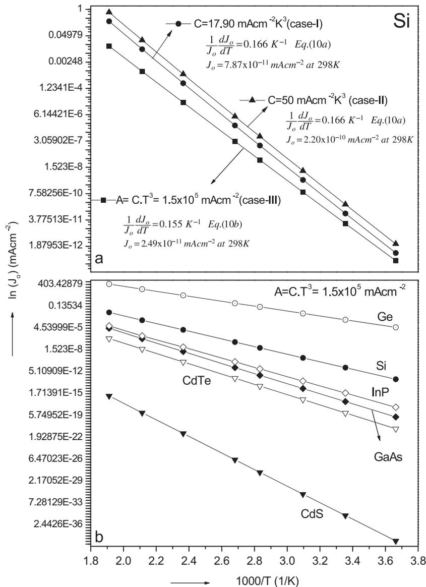
Fig. 2. Arrhenius plots of  $J_o$  in the temperature range 273–523 K: (a) for Si solar cells for three cases: (I)  $C=17.90 \text{ mA cm}^{-2} \text{ K}^3$  (Eq. (9a)) [21], (II)  $C=50.0 \text{ mA cm}^{-2} \text{ K}^3$  (Eq. (9a)) [24] and (III)  $A=C.T^3=1.5 \times 10^8 \text{ mA cm}^{-2}$  (Eq. (9b)) [22]. (b) for solar cells based on Ge, Si, InP, GaAs, CdTe and CdS for case (III).
