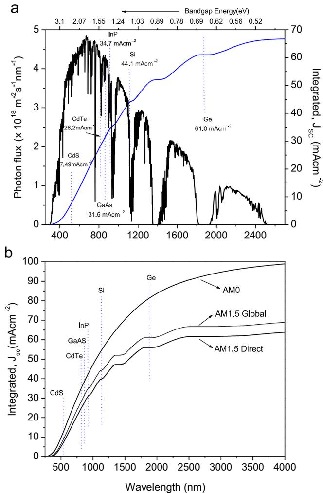
**Fig. 3.** (a) Photon flux from the sun at the earth's surface ( $1000 \text{ Wm}^{-2}$ , AM1.5G) and the integrated short circuit current density as a function of wavelength (bandgap—top x axis). The integrated  $J_{sc}$  is shown on the right y-axis. (b) variation in maximum achievable  $J_{sc}$  for AM0, AM1.5 D and AM 1.5G spectra with wavelength.
